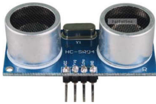
Gambar 4.7. Sensor Ultrasonik SR HC-04 (Sumber : www.google.com )
